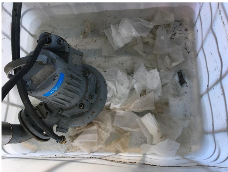
Figure 3: Wet wipe pump clogging test setup
